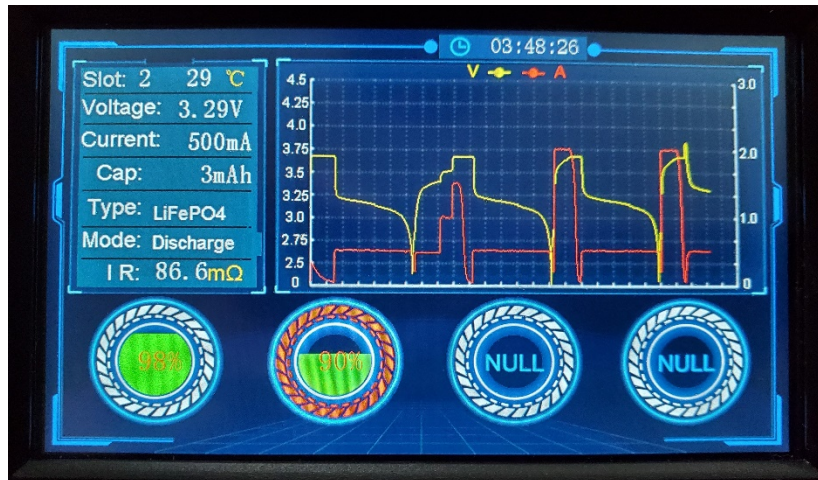
Figure 3: Sample data from cell testing of a LFP battery showing charge/discharge cycling
